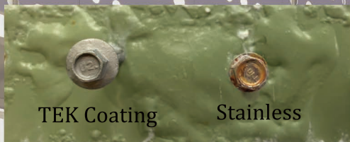
[After 1000 hr Salt Spray Test]
